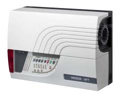
VESDA VFT-15 detectors are multi-channel microbore air-sampling systems with an alarm sensitivity range from 0.001% to 20% obscuration/m (0.0003% to 6.10% obscuration/ft). These detectors are classified as Very Early Warning Smoke Detectors and can reliably detect fire at an early stage, and low to high concentrations of smoke. As a multi-channel system, the VFT detector is able to divide a protected space into sampling sectors, enabling the localization of a fire for faster incident response.
